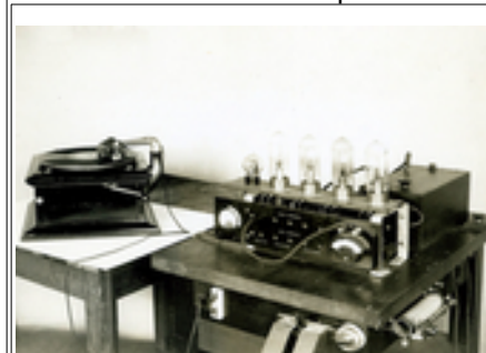
A c1920 WWV transmitter, built by National Bureau of Standards staff and coupled with a hand-crank record player. [Photo courtesy of WWV/NIST]
